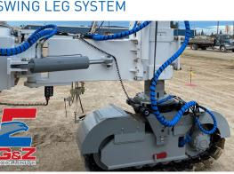
The **SmartLeg** system in tandem with **AccuSteer** allows the swing leg angle to be adjusted on-the-fly to maneuver around an obstacle while automatically keeping the crawler track straight ahead.
