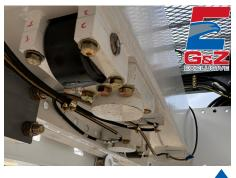
The VariWidth system features cam rollers with optional hydraulic clamping pucks to quickly and easily extend and retract the telescopic tractor frame for width change. The cam rollers are adjustable to remove any frame deflection.
