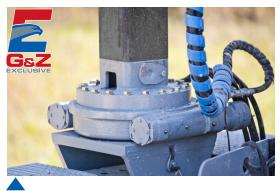
The **AccuSteer** system using hydraulic motor driven slew drives with 320 degree rotation offers unparalleled maneuverability and accuracy, allowing synchronized steering in 90 degree mode in every swing leg position.
