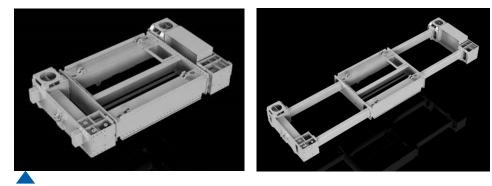
The patented VariWidth, double telescopic tractor frame, with single stage telescoping per side, allows 14ft (4.27m) of telescopic ability, the widest range in the industry. This is made possible by G&Z's patented tunnels through the bolsters. The heavy duty construction along with adjustable cam rollers and optional hydraulic clamping pucks ensures the tractor frame is rigid and without deflection.
