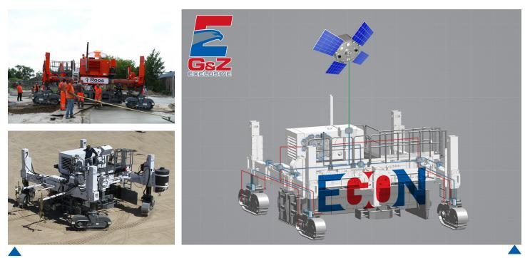
EGON semi-automatically reconfigures the paver into 90 degree, counter-rotation, and transport mode saving time and money.
