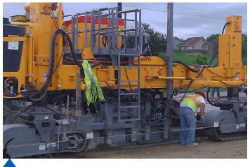
As an option, Guillotine Sideforms with -2 to 18" (-50 to 457mm) of hydraulic adjustment can be supplied split, allowing independent adjustment of the front and rear portions of the sideform. The rear half of the sideform is equipped with hydraulic open / close cylinders which are powerful enough to close against plastic concrete.
