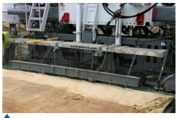
For extra smoothness, the S600 can be fitted with G&Z's optional Trailing Finishing Pan (TFP). The 48 in. (1.2m) wide TFP with fixed edger pans provides a proven method of finishing the pavement surface with fine adjustment, ensuring sharp edges. It also accommodates a wide range of side bar inserters.
