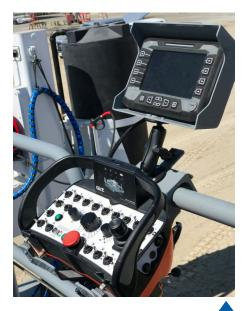
EGON Belly Pack console provides great flexibility to the operator. The Belly Pack includes a relocatable docking station for the belly pack and the operator display.
