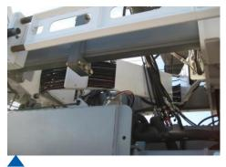
Each side of the the tractor frame is provided with a hose hinge matching the 7ft (2.13m) of telescopic ability of the frame per side.
